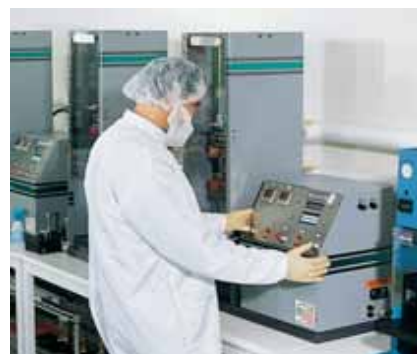
Carver Auto "C" presses molding medical components.*
