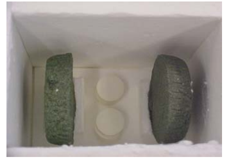
SiC-70 Thermcepts™ in an RMS Thermal Box™ with zirconia (ZrO 2 ceramic) pellets to be sintered
